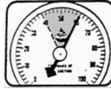
**40 - 60 Centibars:** For clayey soil there is still adequate soil moisture. For loamy and sandy, irrigation should be started.
