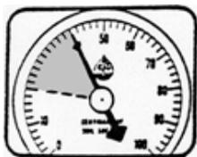
**20 - 40 Centibars:** For clayey and loamy soils, no irrigation is needed. There is adequate soil moisture and aeration. For sandy soils, irrigation should be started.
