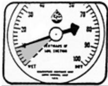
**0 - 10 Centibars:** The soil is saturated with water. No irrigation should be applied. If this condition persists for more than a few weeks during
