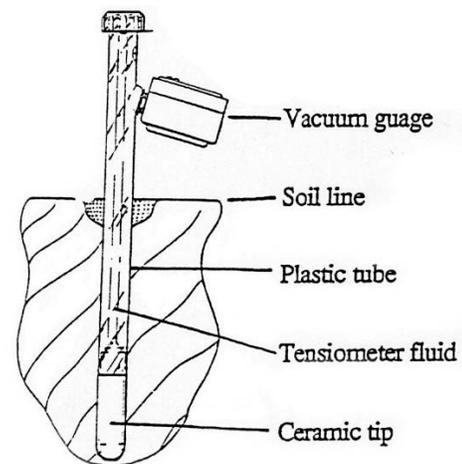
Care should be taken in tensiometer placement so that mowers, people or vehicles do not hit it. Once installed, the tensiometer should remain in place for as long as the moisture needs to be monitored in that area. It must, however, be removed before subfreezing temperatures.
