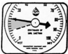
**10 - 20 Centibars:** This range is referred to as 'Field Capacity'. No irrigation is necessary. There is adequate moisture and air at this level to provide plant growth.
