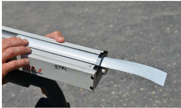
Figure 3: Graph paper that records measurements being loaded into the resistograph
