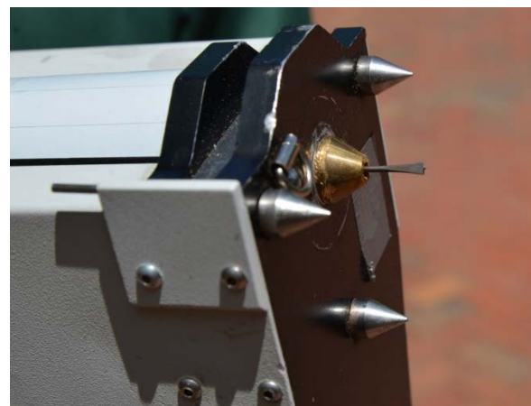
Figure 2: Close-up of drilling needle
