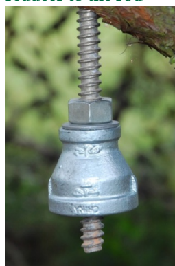
Figure 7: Attach the reducer to the rod
