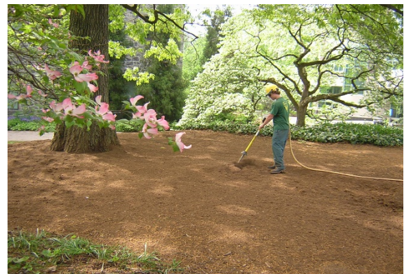
Figure 1: An AirSpade® being used to loosen soil for a shade garden planting
