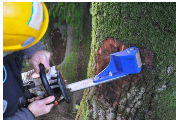
Figure 1: Power planer used to rapidly excise bark tissue
