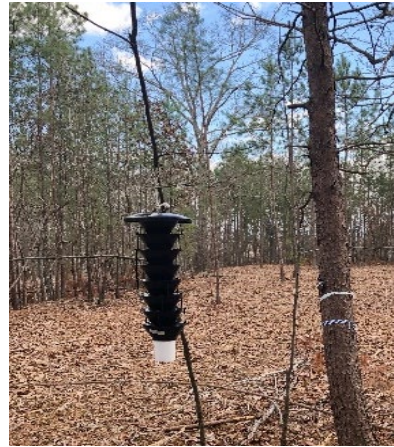
Figure 3: Bark beetle funnel trap used in a push-pull management strategy
