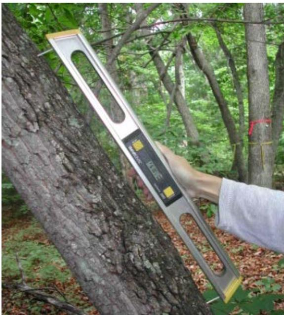
Two nails are driven in the trunk, either the front or backside of the lean, along the length of the trunk. Good nails to use are long aluminum siding nails such as Homeshield Hy-Tensil 2 ¼ x 0.128 inch (Forestry Supplier 79285). The nails should be hammered a quarter to a half inch (0.5-1.2 cm) into
