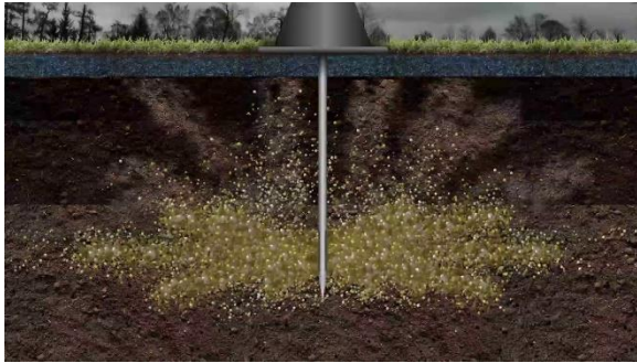
Figure 2. Air and porous particle injection under soil surface. (Image credit: VOGT)
