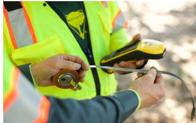
Figure 1: Bartlett Inventory Solutions uses Trimble® 24-channel GPS receivers to collect location and attribute information in the field
